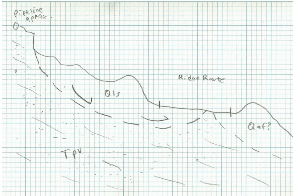
Figure 6 – Inferred Landslide Cross Section within the Peace Valley Fm (Tpv). Not To Scale.
